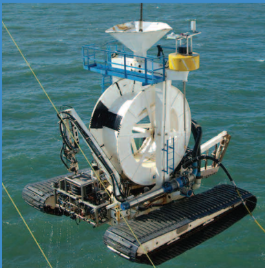
Remotely operated vehicle used for cable burial
