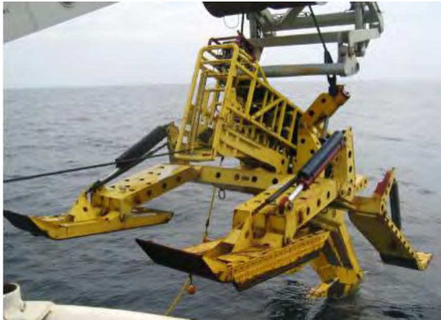
Figure 22. Typical sea plough
