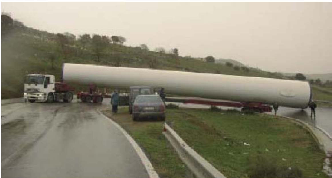
Picture 3.5 Road transportation of a wind turbine tower part
