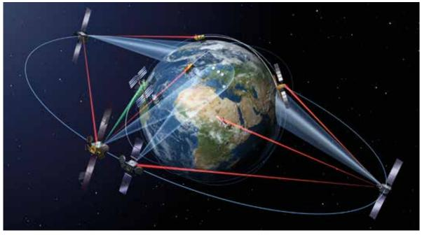
Figure 23: Schematic of the European Data Relay System (EDRS)<sup>48</sup>
