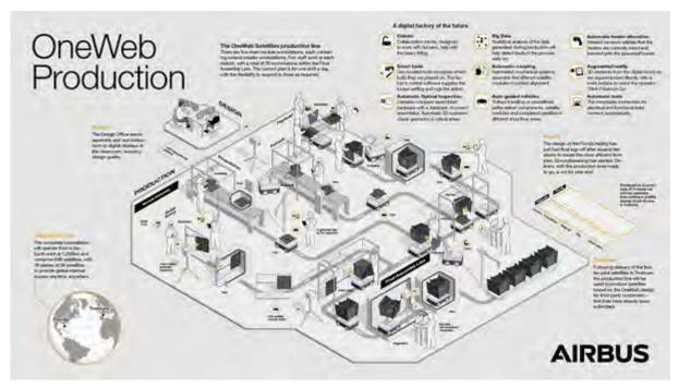
Figure 61: OneWeb and Airbus manufacturing process<sup>134</sup>
