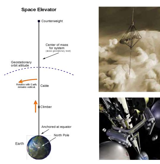
Figure 114: A space elevator concept using a tether made out of e.g. carbon nanotubes<sup>215</sup>
