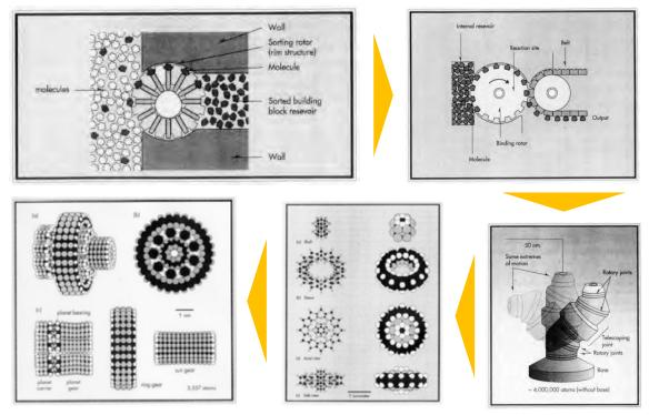
Figure 115: Schematic of a production of a molecular planetary gear with a single atom<sup>216</sup>
