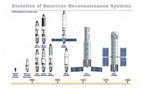
Figure 124: Size comparison of US spy satellite systems<sup>238</sup>
