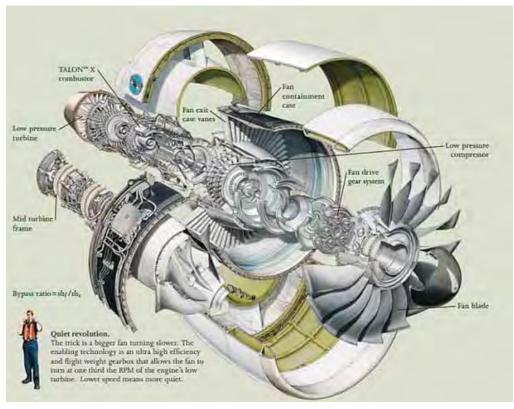
Figure 99: Pratt & Whitney's GTF engine, using a planetary reduction gear to reduce the speed of the fan, will power the new A320neo<sup>193</sup>
