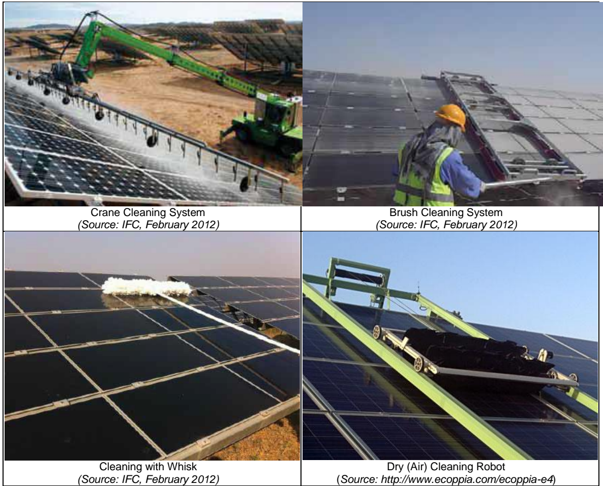
Figure 8.9. Sample Photographs of Different Photovoltaic Panel Cleaning Systems
