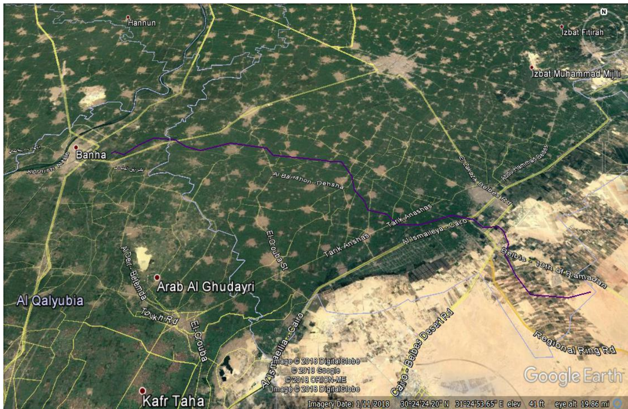
Figure 1-2: Route of 500kV from 10th Ramadan SS to East Banha power plant
