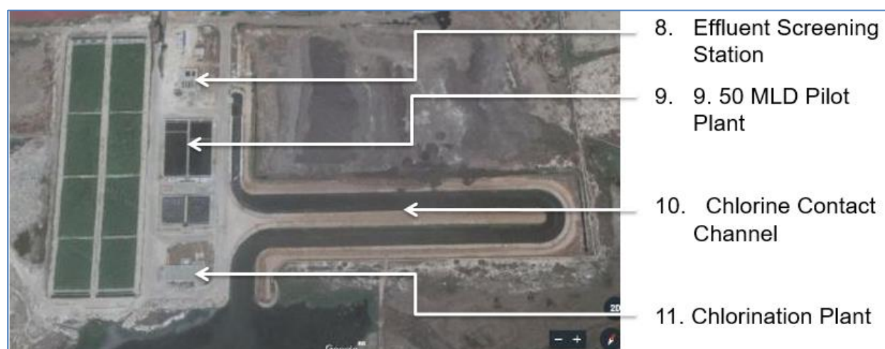
Figure 5: Layout of existing treatment facilities (continuation)
