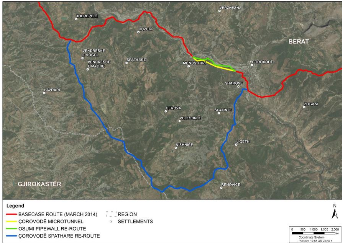
Figure 4-8: Corovode Re-route Alternatives
