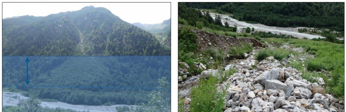
Typical situation of a alluvial/colluvial fan which will be submerged by the reservoir and subject to reservoir draw-down (left) and soil structure of such a fan, composed of large-scale granular material (cobbles to blocks) in a sandy-gravelly matrix (right).
