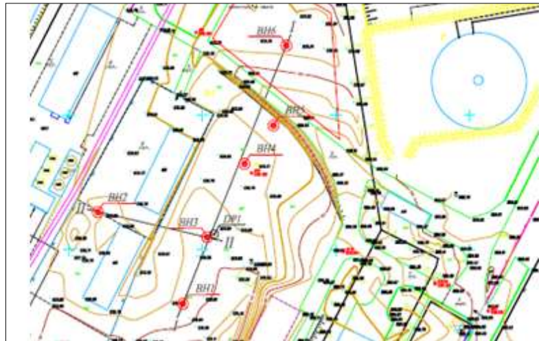
FIGURE 4.3-2 LOCATION OF THE INVESTIGATION DRILLING AT THE SITE OF TPP SOFIA (ACCORDING TO DATA FROM ECOProCONSULT, 2013)
