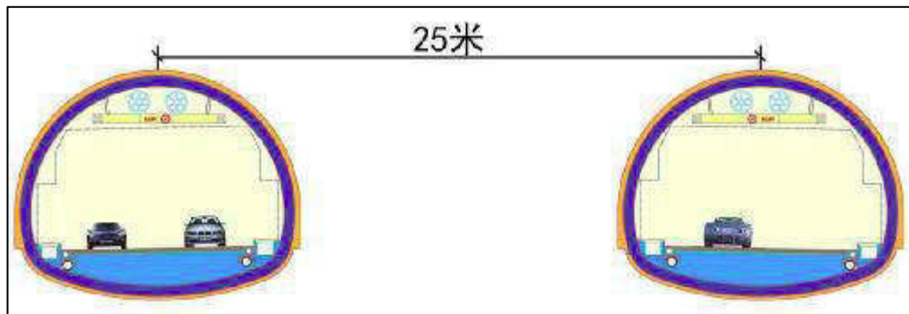
Figure IV-55: Alignment of sub-tunnels of Yufeng Tunnel (SY)
