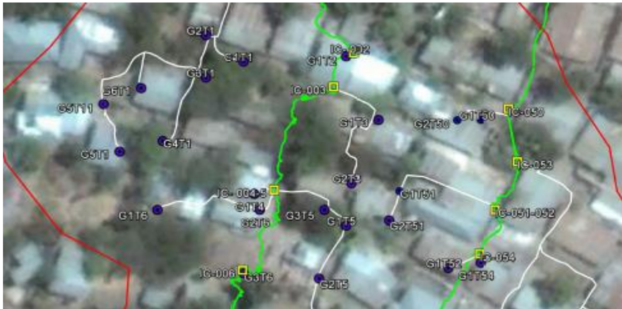
Figure 2-3. Lay-out drawings of the simplified sewerage system to be installed in Nyamanoro Pilot Site (detail)
