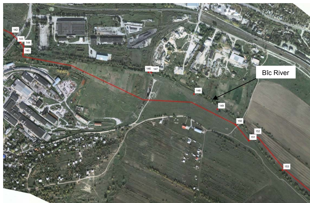
Figure 6-2: Optimization of the route Option 1 between points 145 and 149 to avoid proximity with industrial buildings, the Bîc river and the damaged water treatment plant (the non-connected red dots correspond to the previous line routing)
