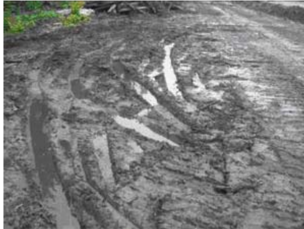
Figure 8-2: Rutting occurring in a wet soil after passage of vehicles (URL 11)
