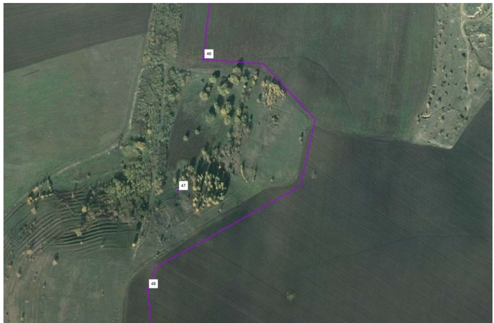
Figure 6-6: Optimization of the common section between points 46 and 48 to avoid passing through a ravine (the non-connected purple dot corresponds to the previous line routing)
