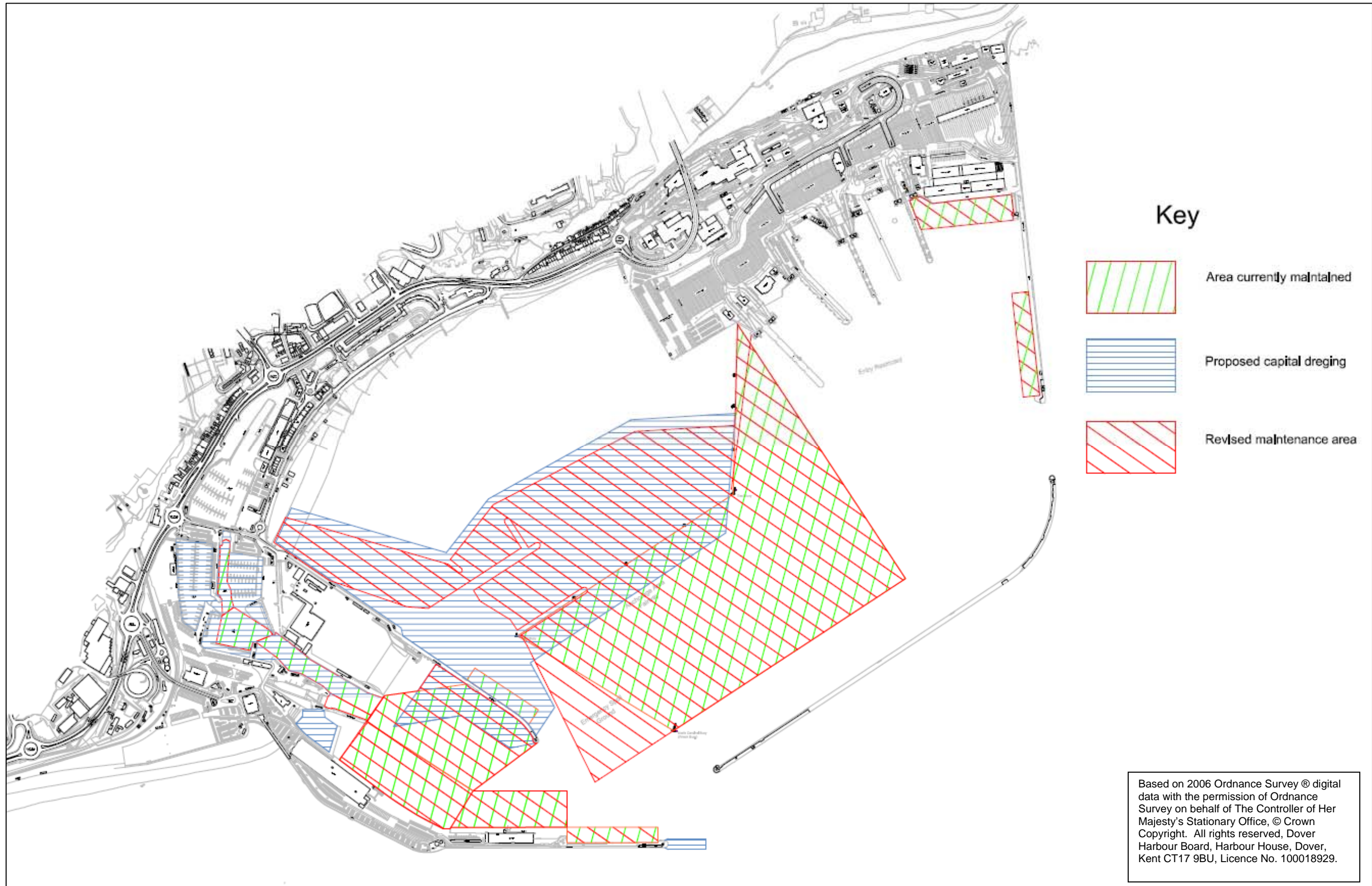
Figure 3.2 Existing maintenance dredge area, proposed capital dredge area and proposed operational phase maintenance dredge area
