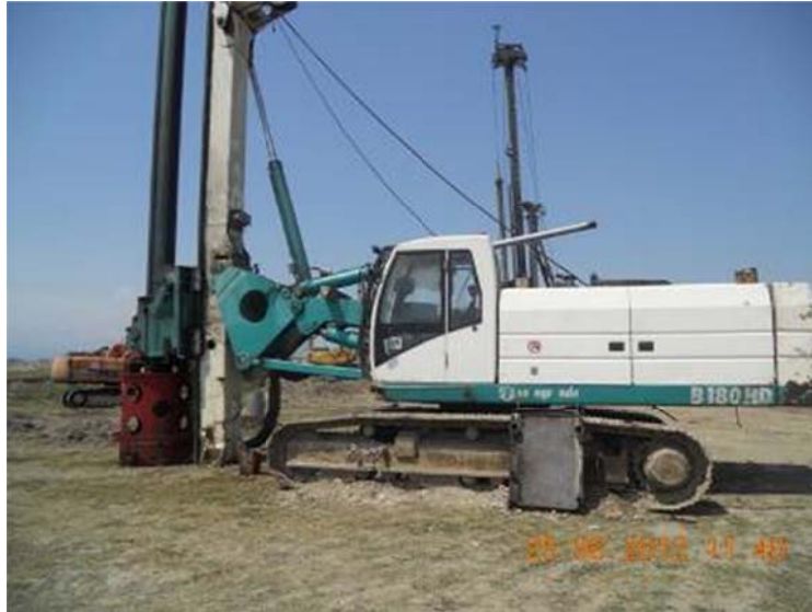
Picture 2.6 Drilling Equipment Widely Used for Pile Arrangement in Georgia
