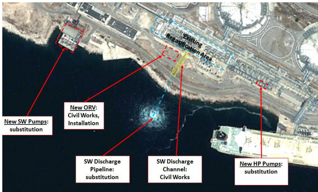
Figure Error! No text of specified style in document..2: Aerial View Sketch of New Equipment Work Areas
