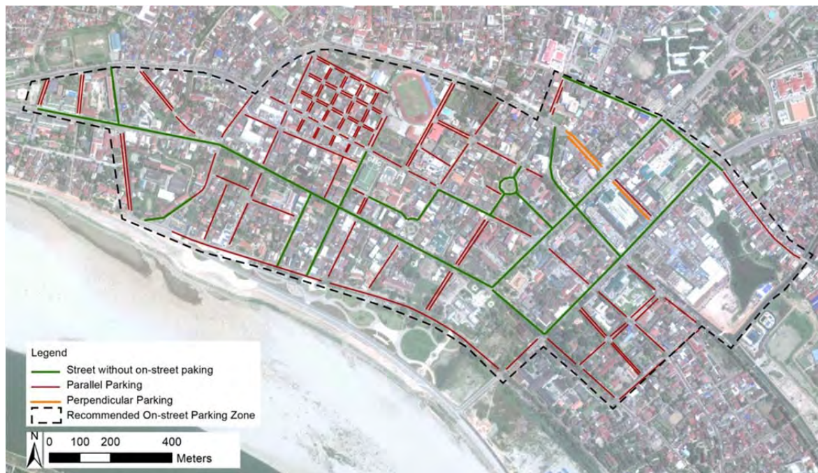
Figure 10. Lay-out of recommended on-street parking zone
