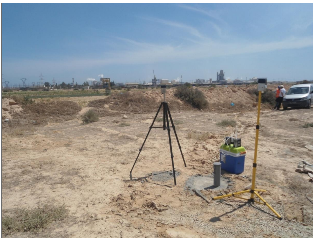
Figure 9 : Measurements of ambient air parameters (near BH3).
