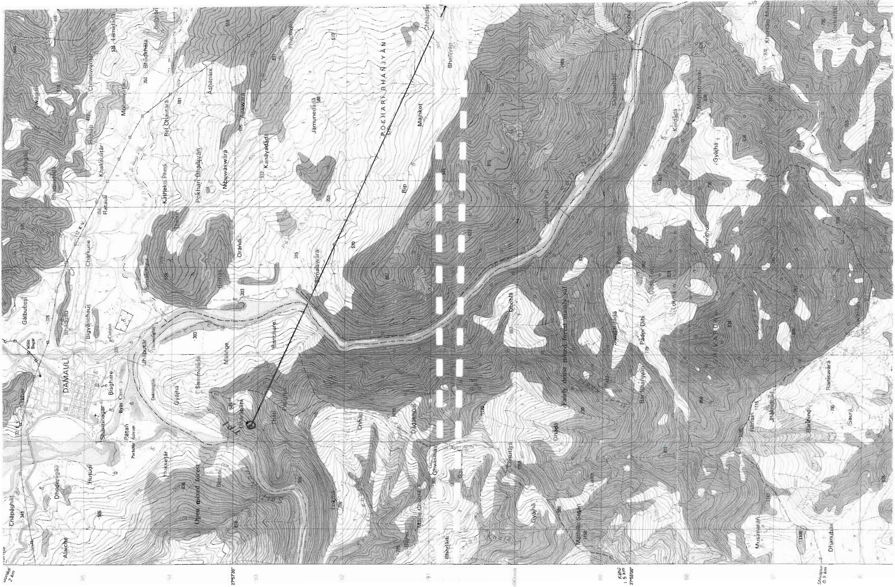
Upper Seti (Damauli)-Bharatpur 220 kV Transmission Line Project Route Alignment Map Scale 1:50,000
