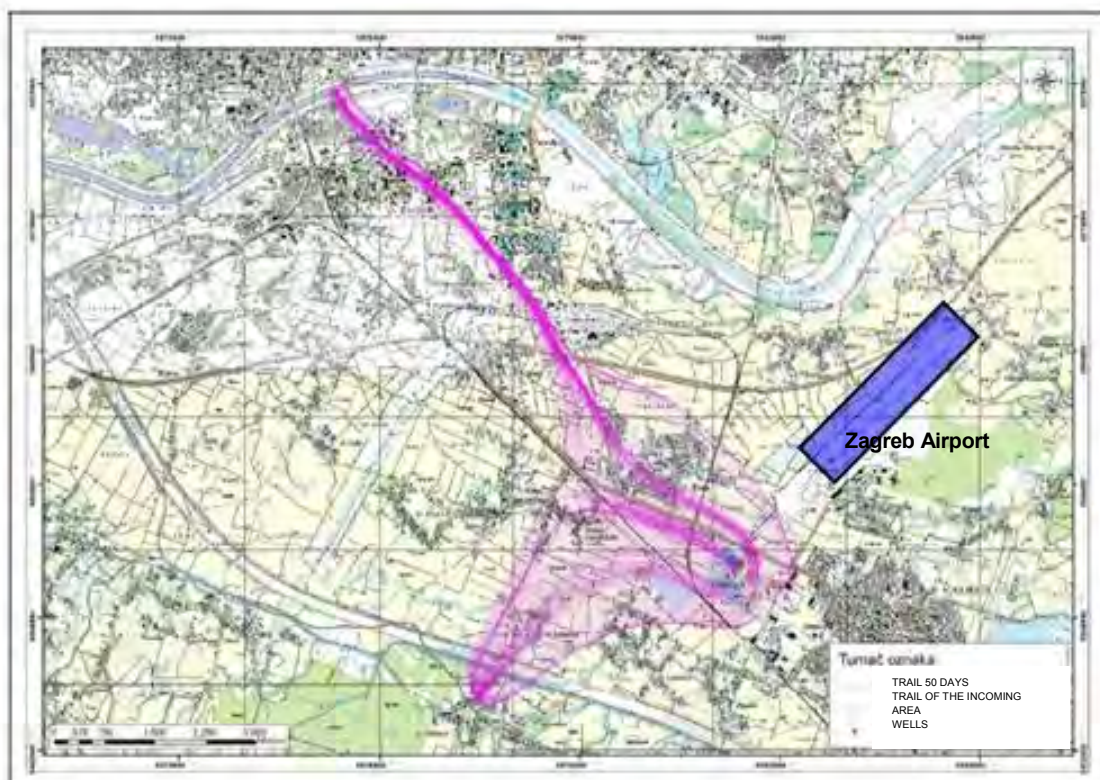
Figure 3.6.-7. Simulated track movements of particle for low water (according to the Study of wellfield protection zones in Velika Gorica, Bačani and Posavec, 2009)
