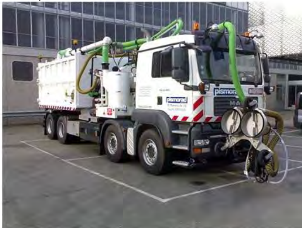
Slika 1.3.10. Cleaning device for cleaning tire marks Stripe Hog 8000
