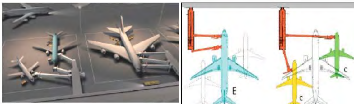
Photo 1.3.2.-1 Flexible use of type E aircraft or two type C aircraft enabling optimum flexibility and efficient use of the available apron area.
