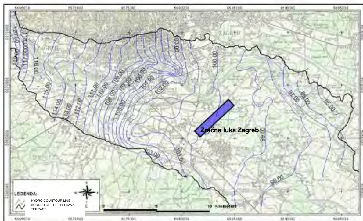
Figure 3.6.-5. Hidroizohipse at low water (07/09/2000) (according to the Study of protection of wellfield zones in the City of Zagreb - I Phase Bačani etc 2005)
