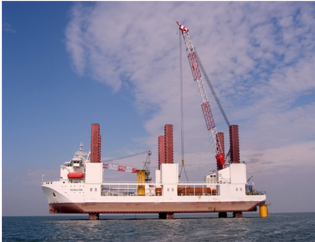
Figure 9: Purpose built windfarm construction vessel (Source: MPI vessel “Resolution”, (Kentish Flats, Elsam))
