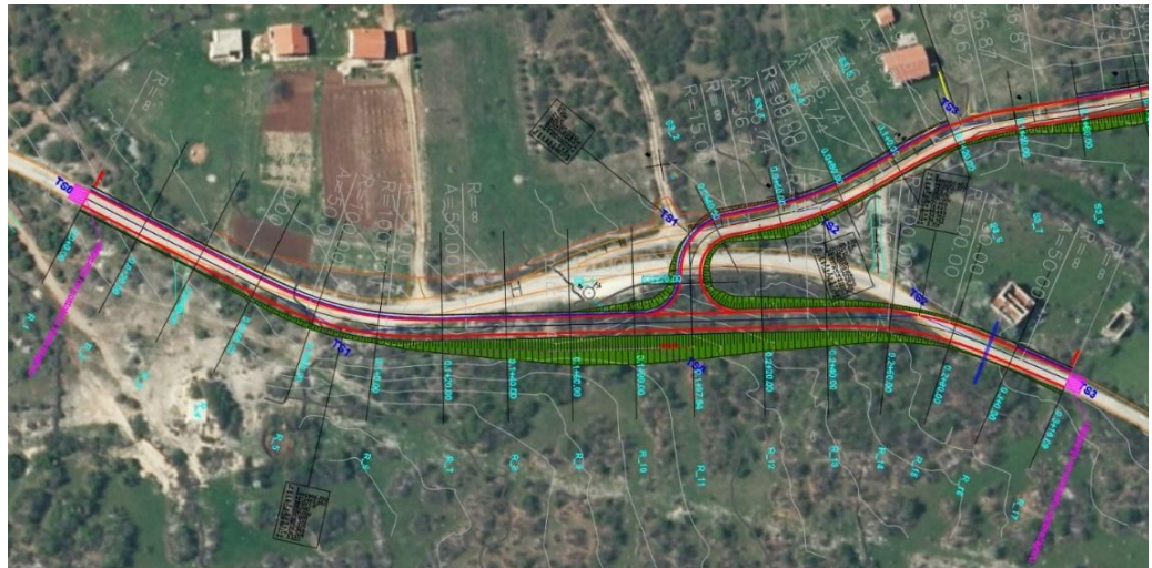
Figure 3-36: Design situation of the section SR3, relocation of the existing road and newly designed T-interchange
