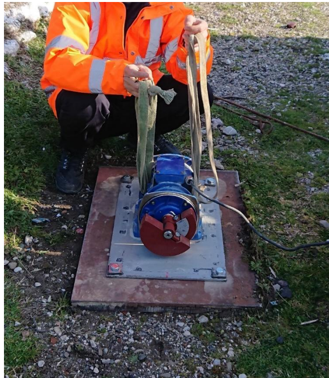
Figure 12-3: 250 kg Vibration generator
