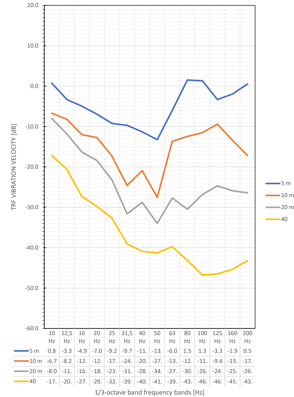
Figure 12-19: Transfer function of measurement points at Site #4
