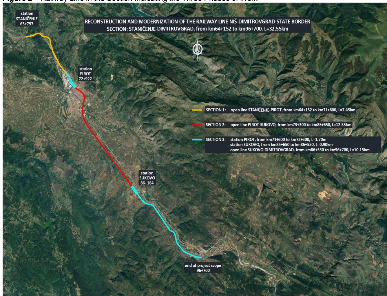
Figure 2 – Railway Line in the Section Indicating the Three Phases of Work
