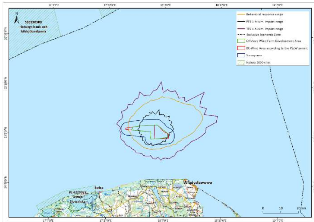
Figure 6.6. Impact range of underwater noise from single pile driving in the BC-Wind OWF Area for the harbour porpoise with the application of an NRS [Source: internal materials]
