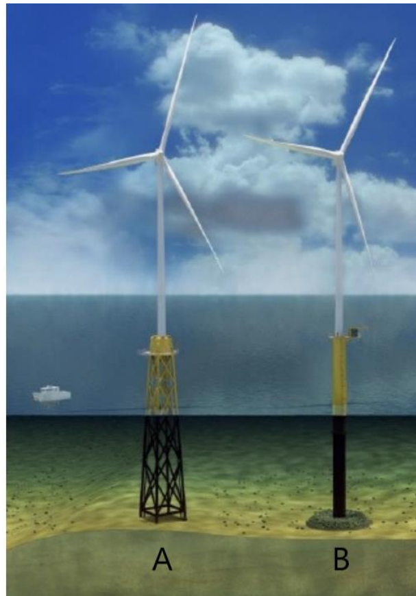
Fig. 3.5. Selected types of support structures with foundations that are permanently bottom-bound: A – truss, B – monopile
