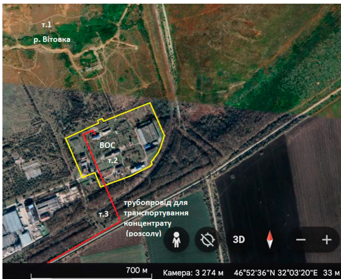
FIGURE 24 - LAYOUT OF THE WTP IN MYKOLAIV AND LAYING OF THE PIPELINE FOR TRANSPORTING CONCENTRATE (BRINE) FROM REVERSE OSMOSIS
