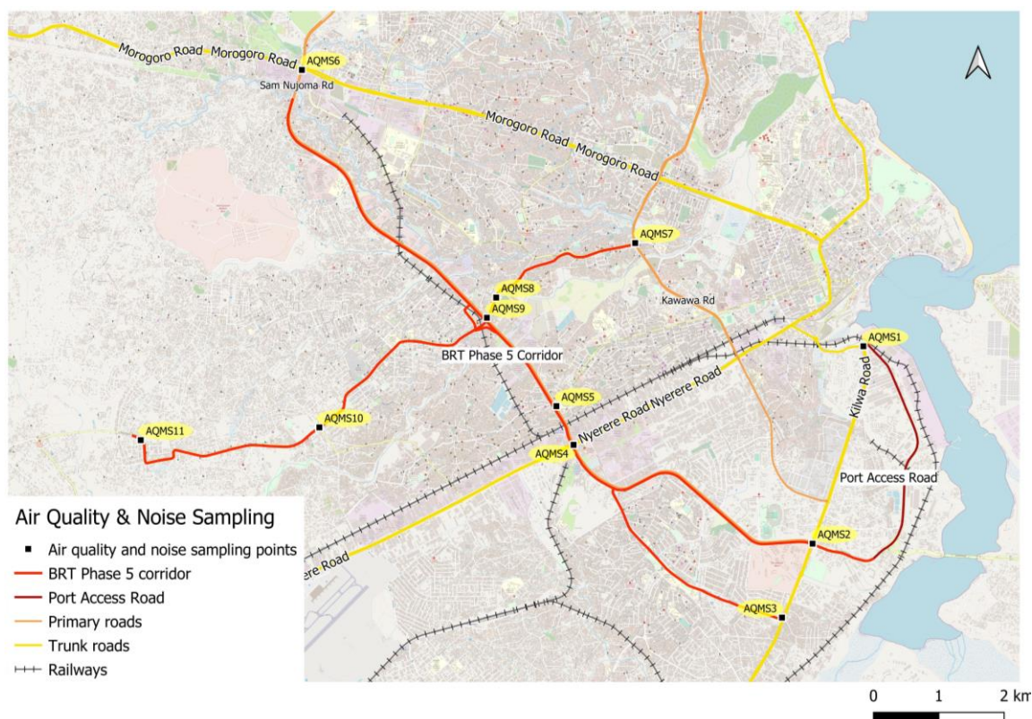
Figure 4-12: Distribution of air quality sampling and noise measurement locations as part of the baseline assessment
