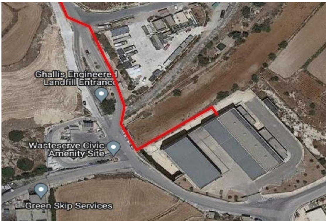
FIGURE 11: CABLE ROUTE (IN RED) FROM ENEMALTA TERMINAL STATION INTO THE ECOHIVE COMPLEX
