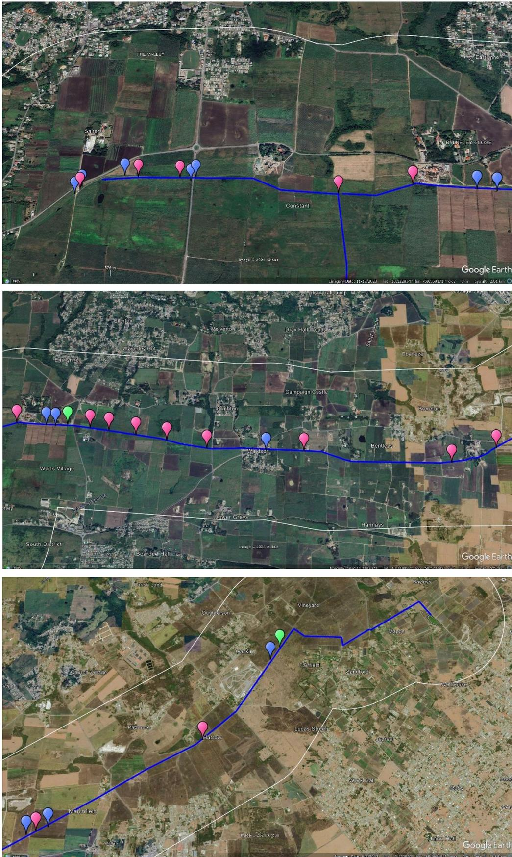
Figure 5-27: Satellite Imagery showing Wells (blue), Bridges (green) and Culverts (pink) from Salters to Bulkeley (top), Carmichael to Carrington (middle) and Carrington to Three Houses (bottom)
