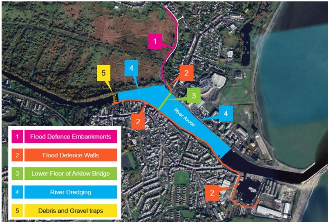
**Figure 4.1:** Overall Layout of Proposed Flood Relief Works
