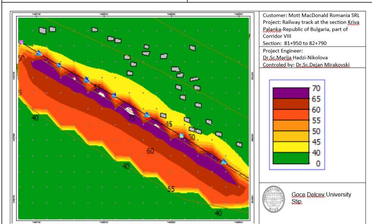
Noise Dispersion Model for section at village of Uzem, once the proposed noise barriers are built
