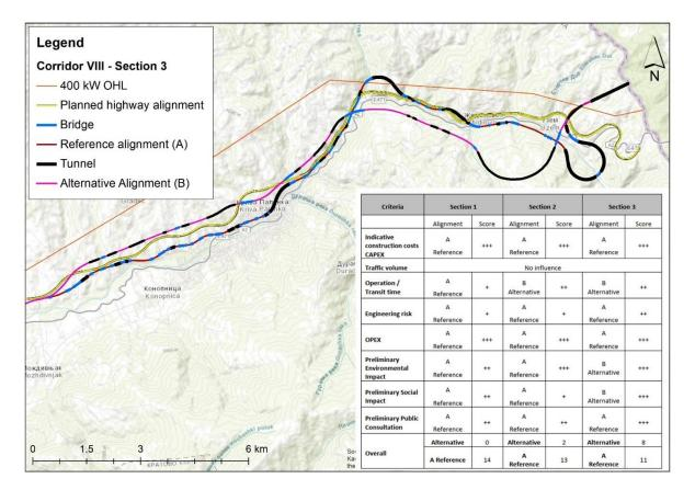
Figure 2 Route of the Reference and Alternative Alignments in Section 3 (Source: Report on Update of the Feasibility Analysis Version C, 16th November 2017)
