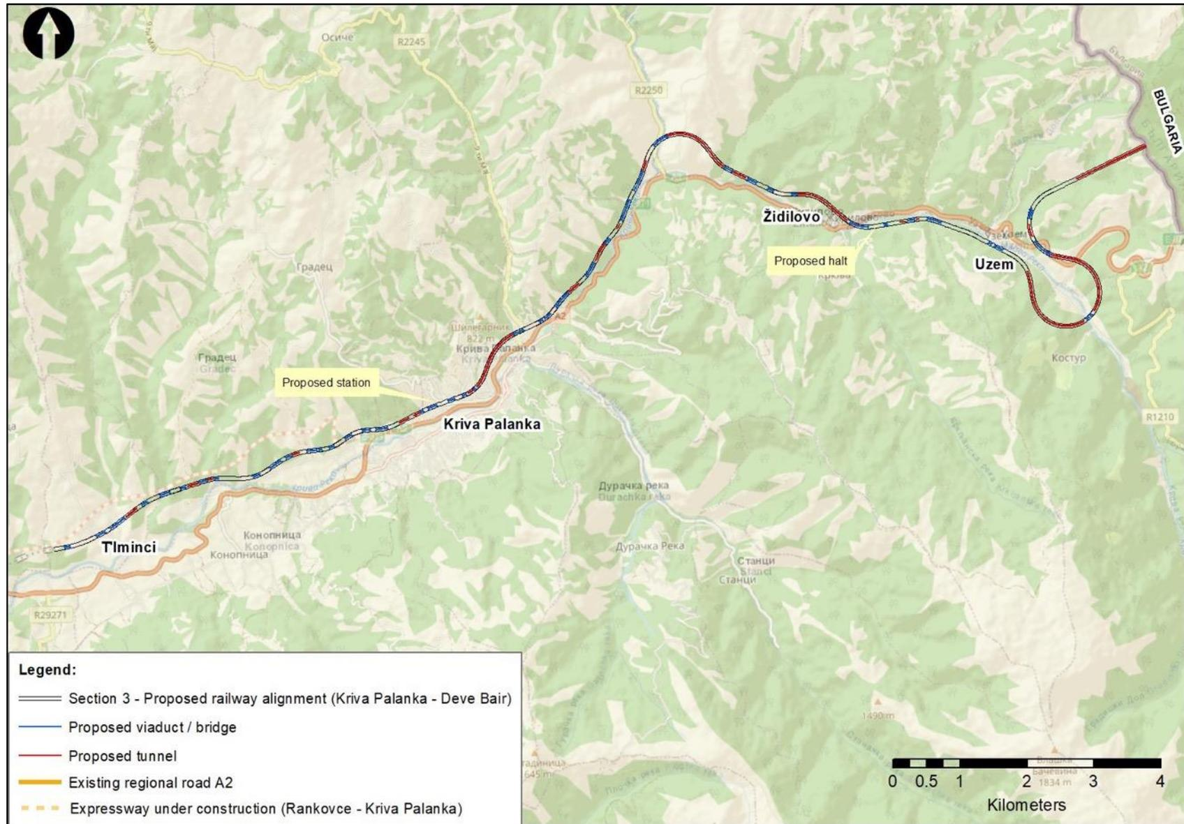
Figure 5 Proposed Alignment of Section 3: Kriva Palanka – State Border with Bulgaria (Deve Bair)
