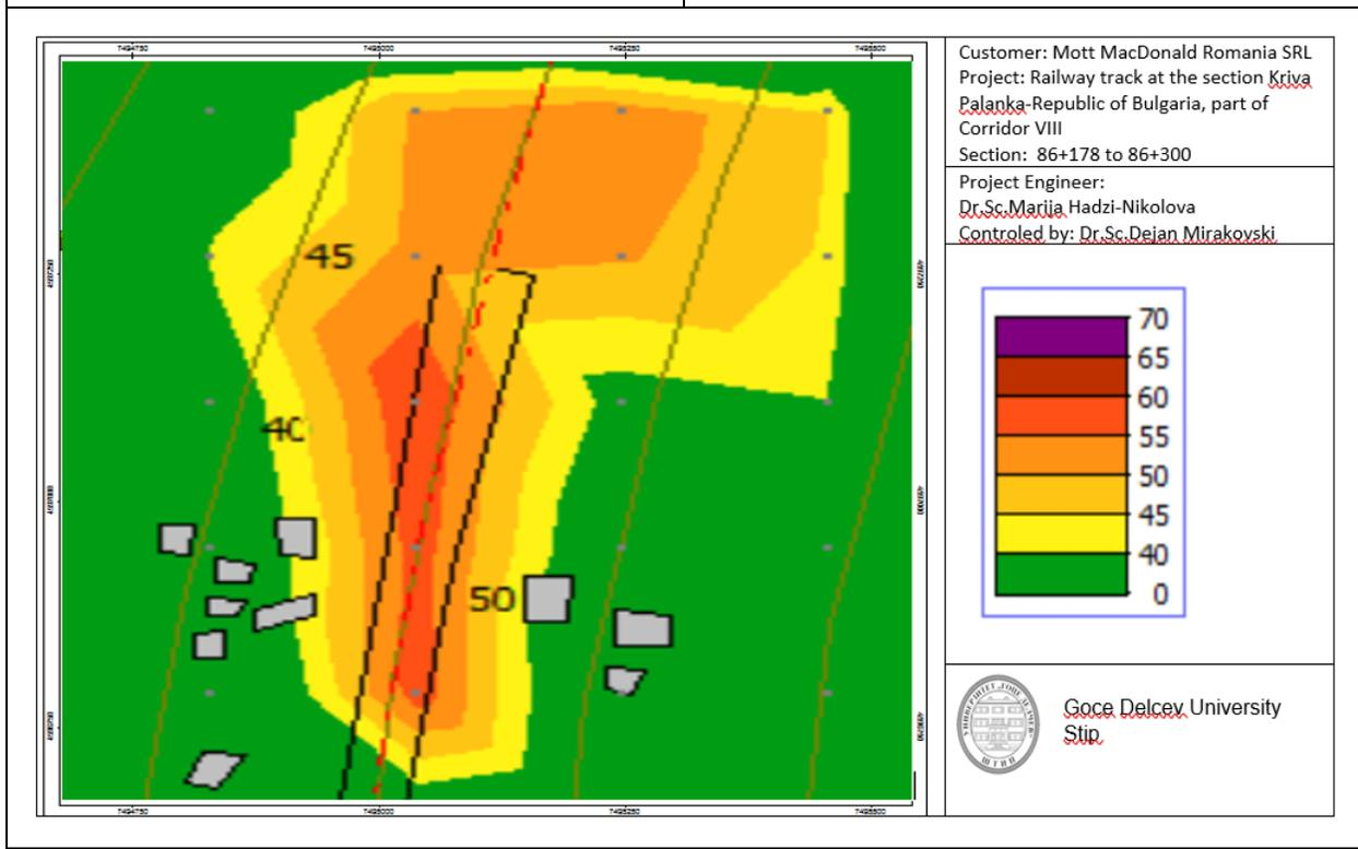
Noise Dispersion Model for section from 86+178 to 86+300 km after at village of Uzem, once the proposed noise barriers are built
