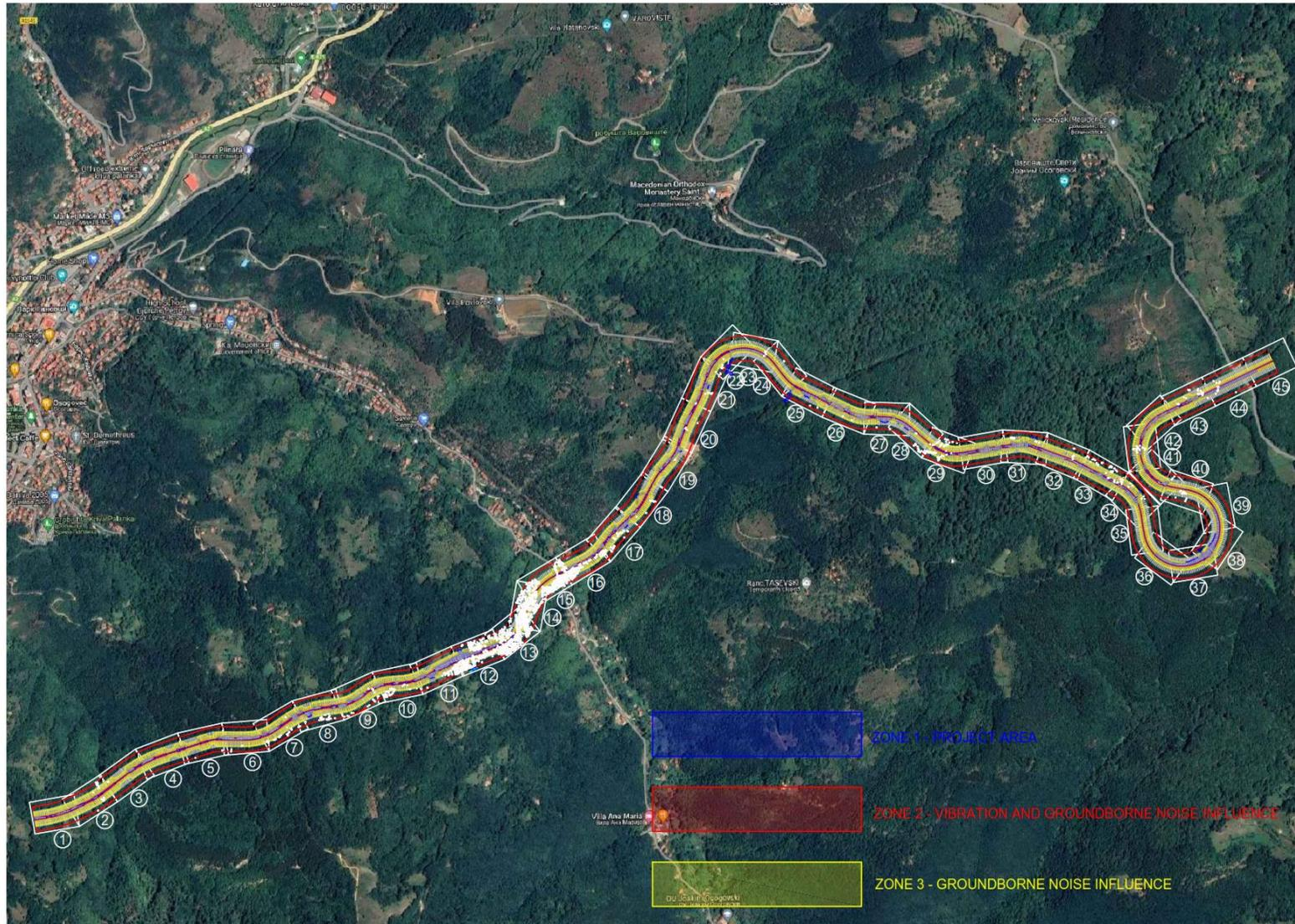
Figure 21 Object locations along the railway corridor with vibration and groundborne noise influence zones
