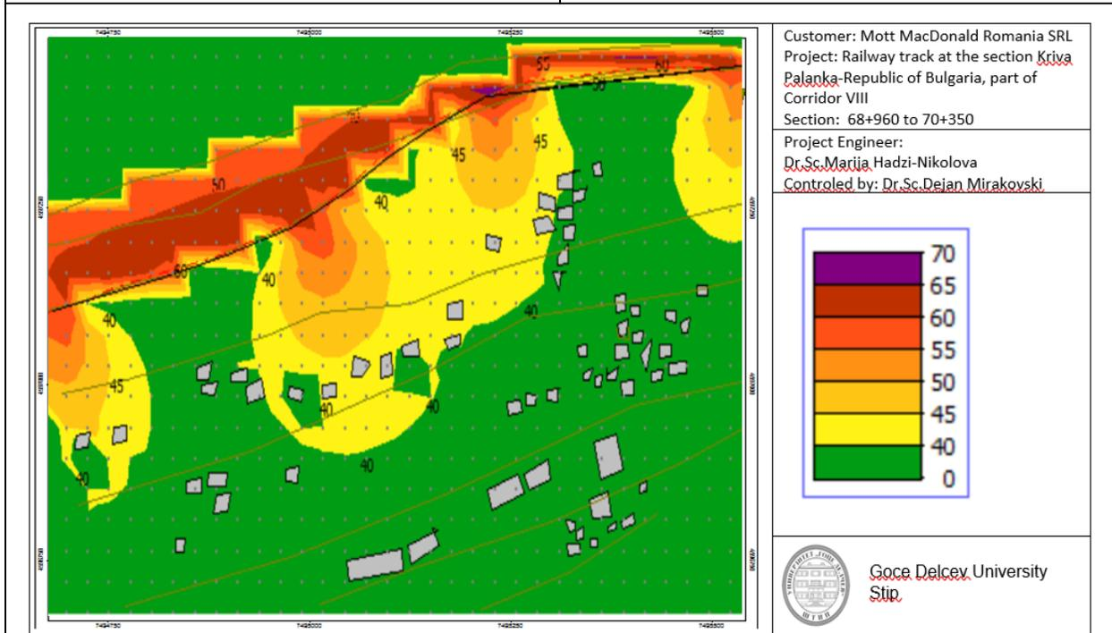
Noise Dispersion Model for section 68+960 to 70+350 before the Municipality of Kriva Palanka, once the proposed noise barriers are built
