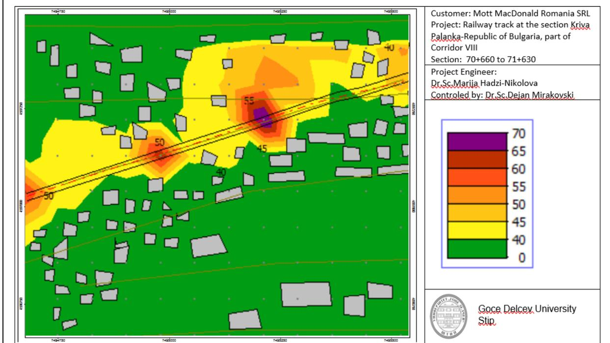
Noise Dispersion Model for section 70+660 do 71+630 at Municipality of Kriva Palanka, once the proposed noise barriers are built
