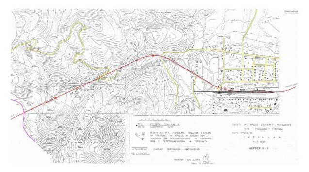
Figure 6 Railway alignment in the territory of the Republic of Bulgaria<sup>6</sup>
