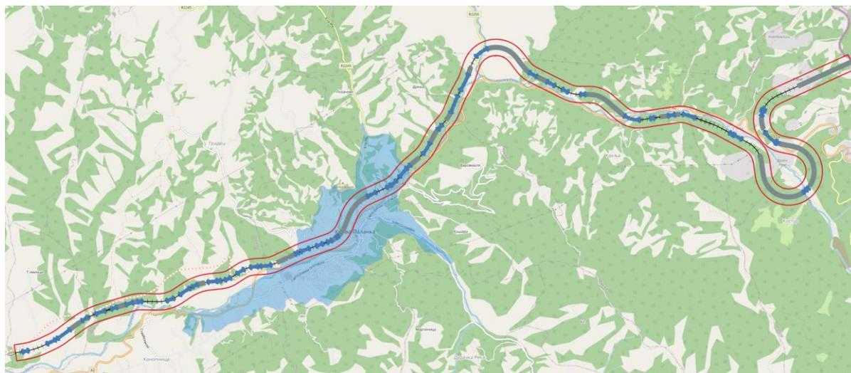
**Figure 20 The position of the railway line with the boundary of vibration impact in relation to the Kriva Palanka settlement**
