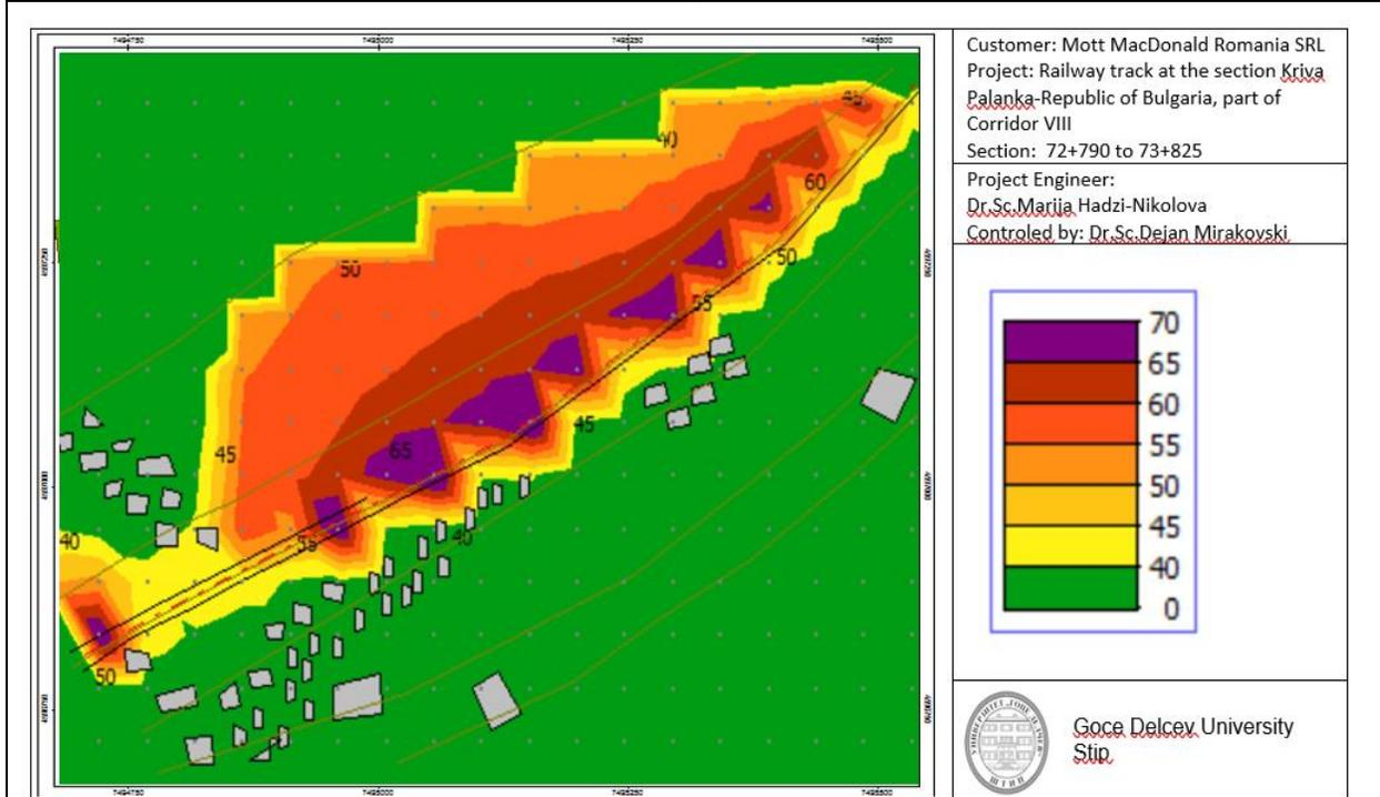
Noise Dispersion Model for section 72+790 to 73+825 at Municipality of Kriva Palanka, once the proposed noise barriers are built
