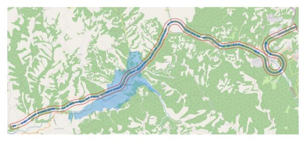
Figure 20 The position of the railway line with the boundary of vibration impact in relation to the Kriva Palanka settlement
