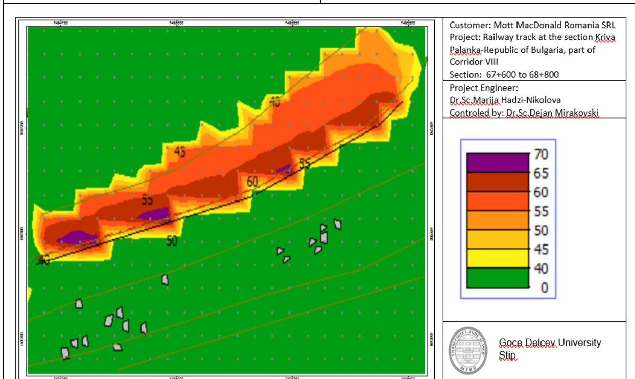
Noise Dispersion Model for section 67+600 to 68+800 before the Municipality of Kriva Palanka, once the proposed noise barriers are built
