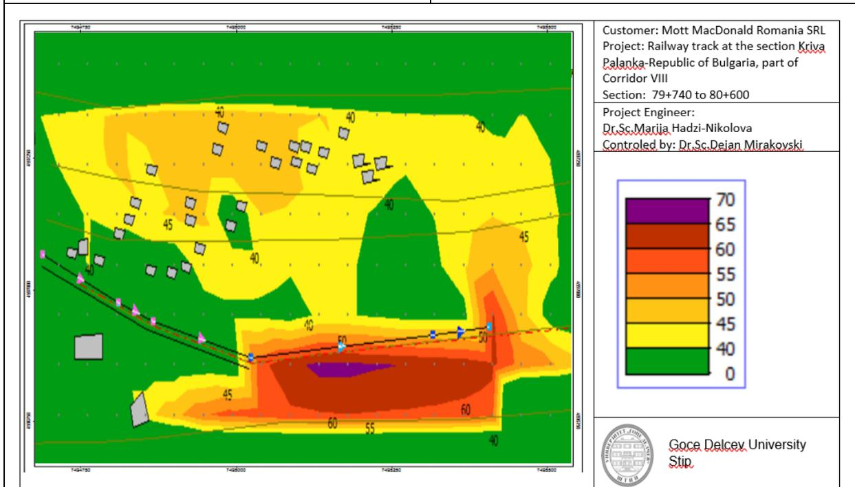
Noise Dispersion Model for section of Zidilovo, once the proposed noise barriers are built
