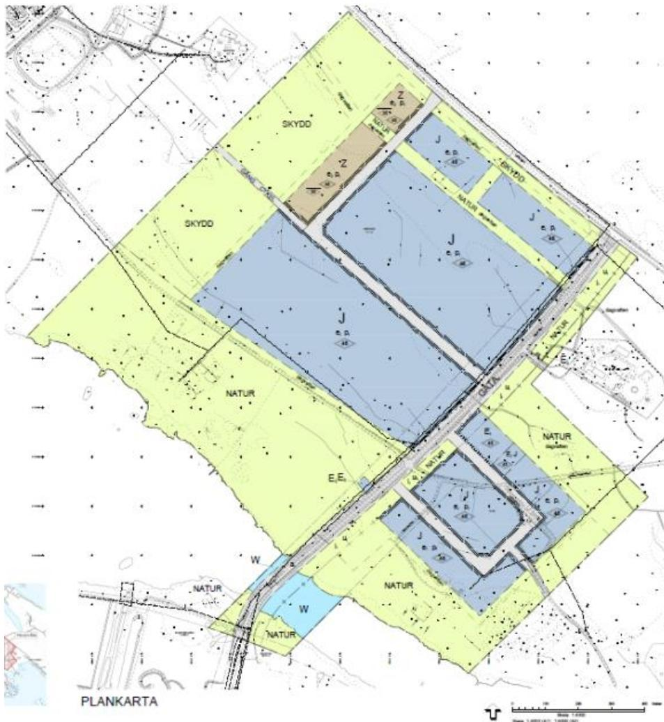
Figure 9. Plan map for detailed planning area for Hertsö field. Green area consists of natural land or protection with certain land reserves for, for example, pipes, while dark blue and brown area consists of planned industrial land. The light blue area, marked with w, marks part of the water included in the plan area.
