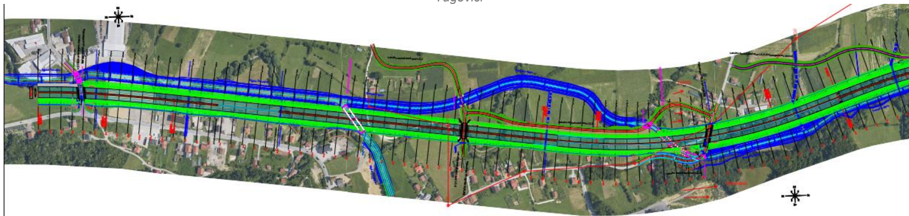
Figure 3: Beginning of subsection Medakovo - Ozimice with regulation of the river Tešanjka and local roads through Medakovo and Trepče to the rest area Tugovići
