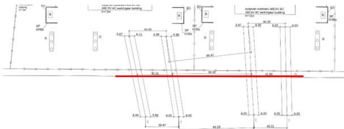
Figure 5.1. The location of the busbars evacuating power from the LPSs and the location of the computational cross-section along which the distribution of the electric and magnetic field was determined
