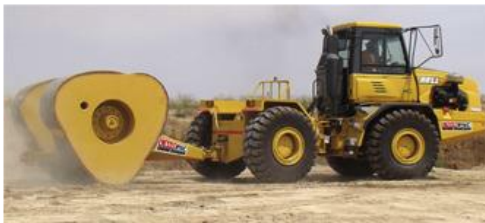
Figure 2-16. Rolling dynamic compaction (RDC)
