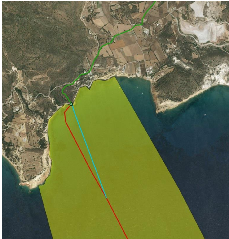
Figure Error! No text of specified style in document.-9 Alternatives considered for scoring the route of the submarine cable in the southern Apple, Regional Unit of Milos (blue-coloured with the first alternative and in red the second alternative — proposed solution)
