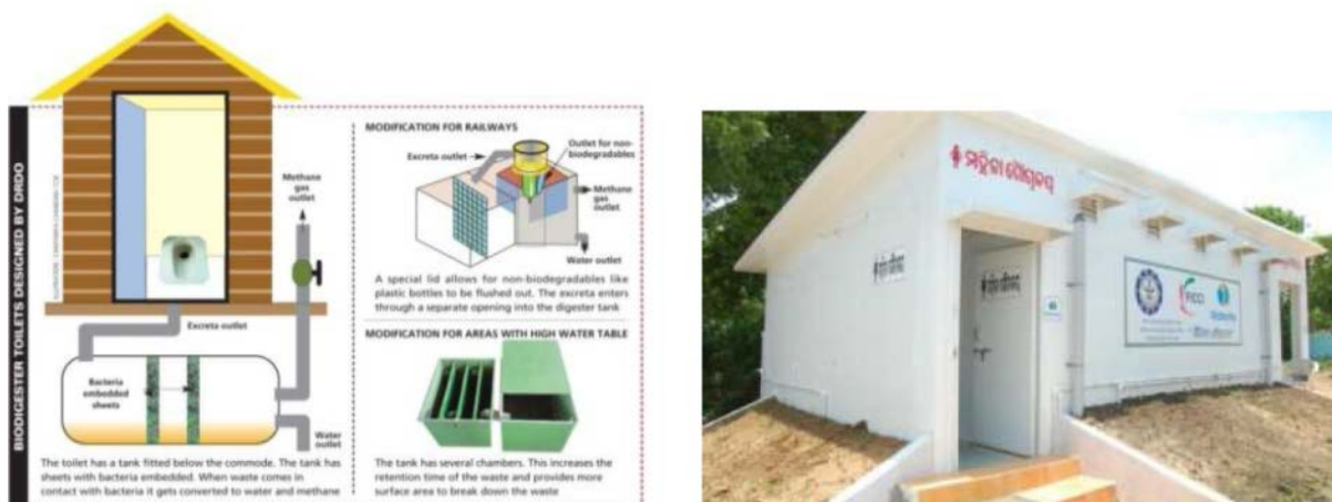
Figure 8.22. Typical Cross Section of Bio Digester
