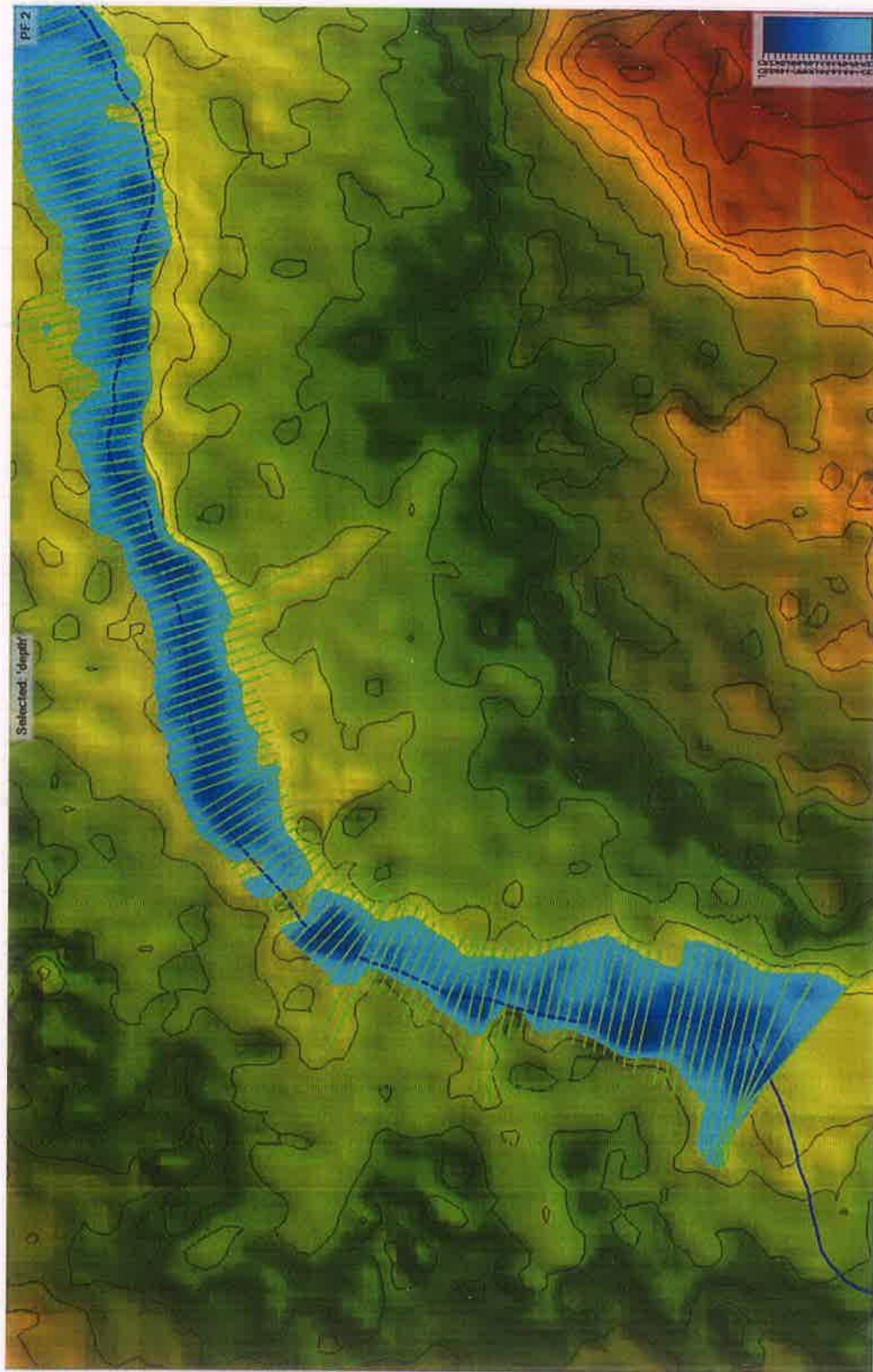
Figure 20: Flood inundation map overlaid SRTM terrain map for the discharge of 1,00,000 ft 3 /s covering reach from Khadakwasla dam to Nanded city
