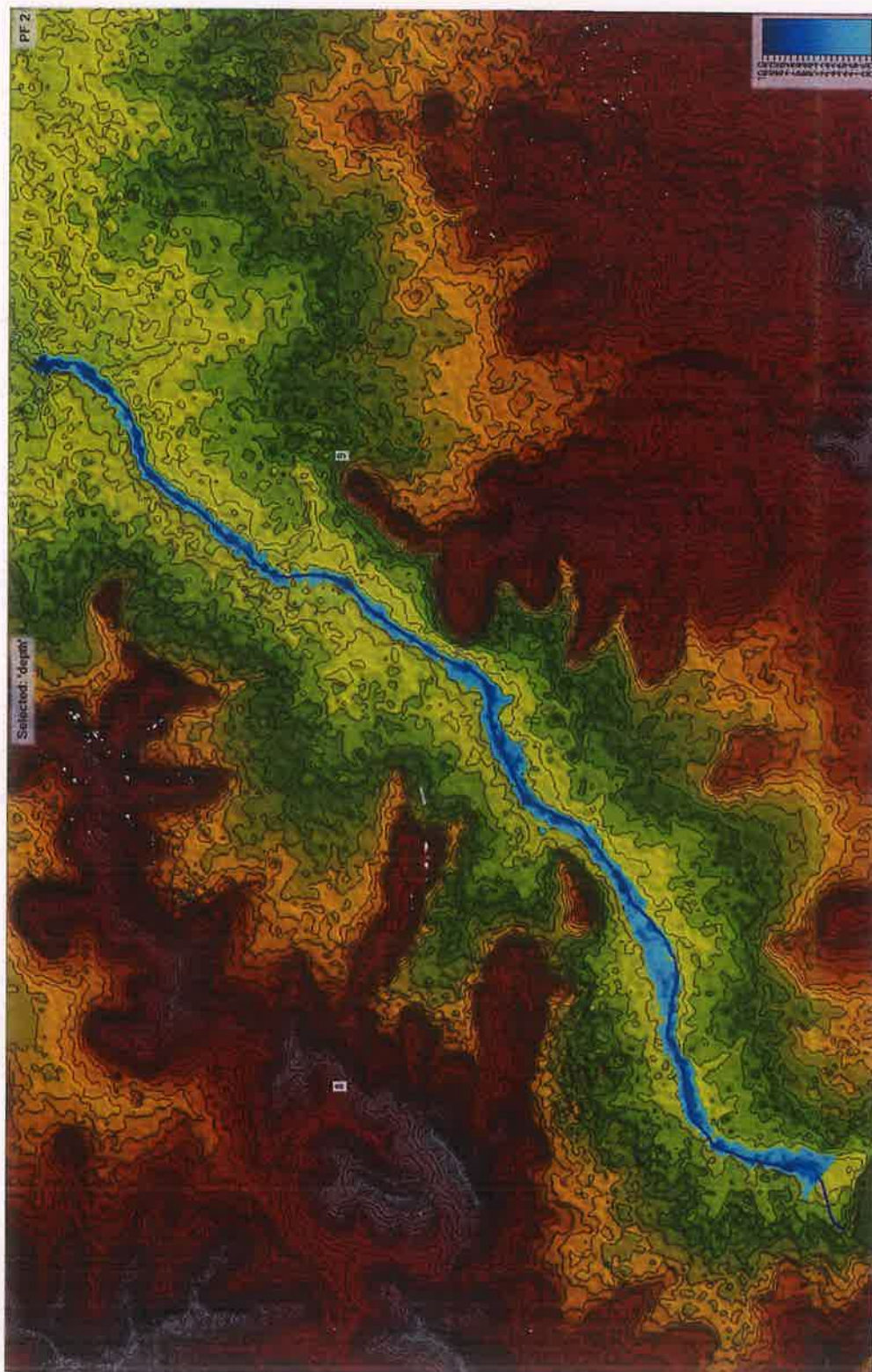
Figure 19: Flood inundation map overlaid on SRTM terrain map for the discharge of 1,00,000 ft 3 /s covering the entire study reach
