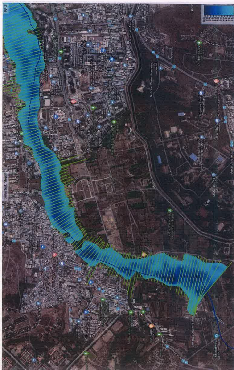
Figure 14: Flood inundation map overlaid on Google map for the discharge of 1,00,000 ft 3 /s covering reach from Khadakwasla dam to Nanded city
