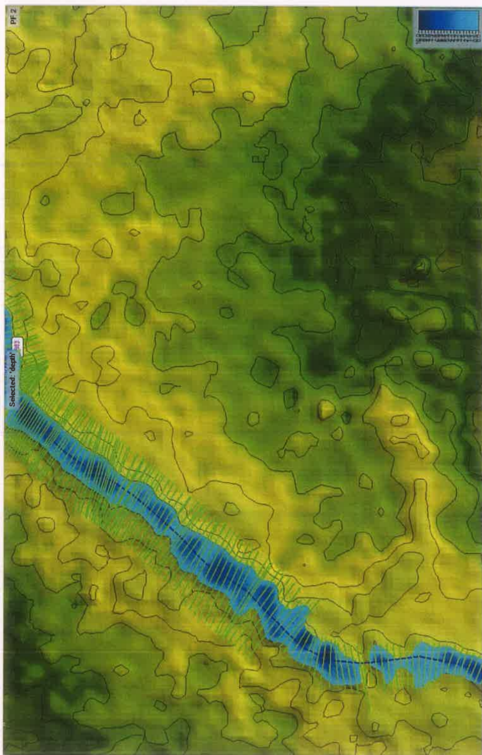
Figure 23: Flood inundation map overlaid on SRTM terrain map for the discharge of 1,00,000 ft 3 /s covering reach from Mhatre bridge to Tilak bridge
