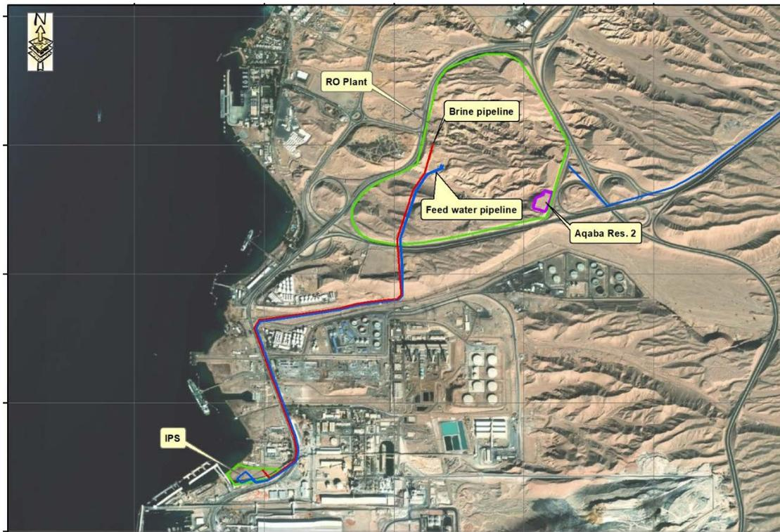
**Figure 2-3: Location of Intake Pumping Station, RO Plant, Feed Water Pipeline and Brine Pipeline**
