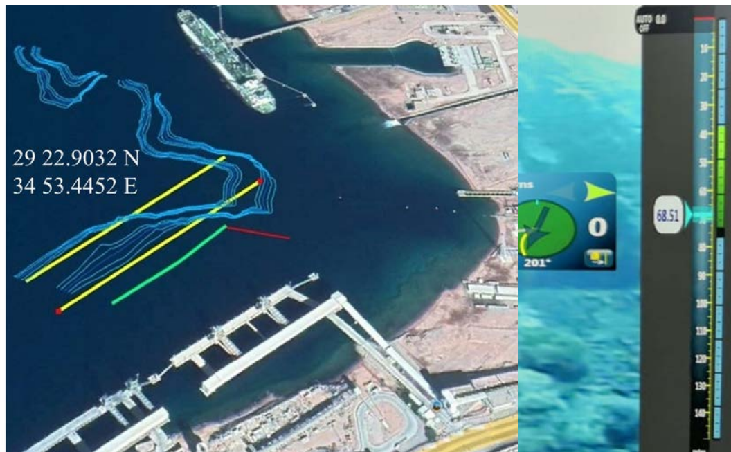
Figure 5-5: Study Site Showing the Two Belts (Yellow) and the Coordinates in the Site (Left). Screen Shot Showing the Depth (68.51 M) at this Moment of the Survey (Right)
