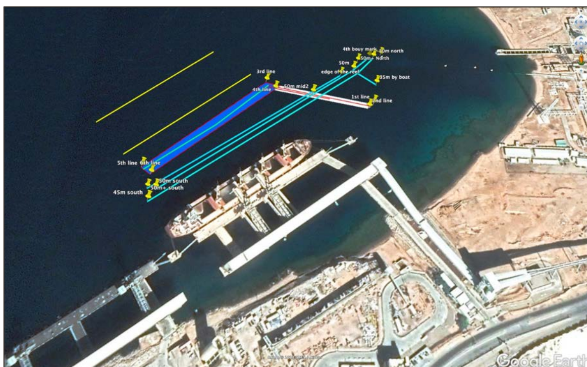
Figure 5-3: Diving Photographic and Video Survey at proposed Brine Discharge Pipeline Path and Diffusers Location
