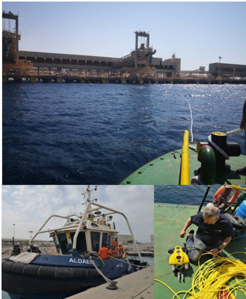
Figure 5-4: The ROV and Boat that Were used to Carry Out the Deep Video Survey
