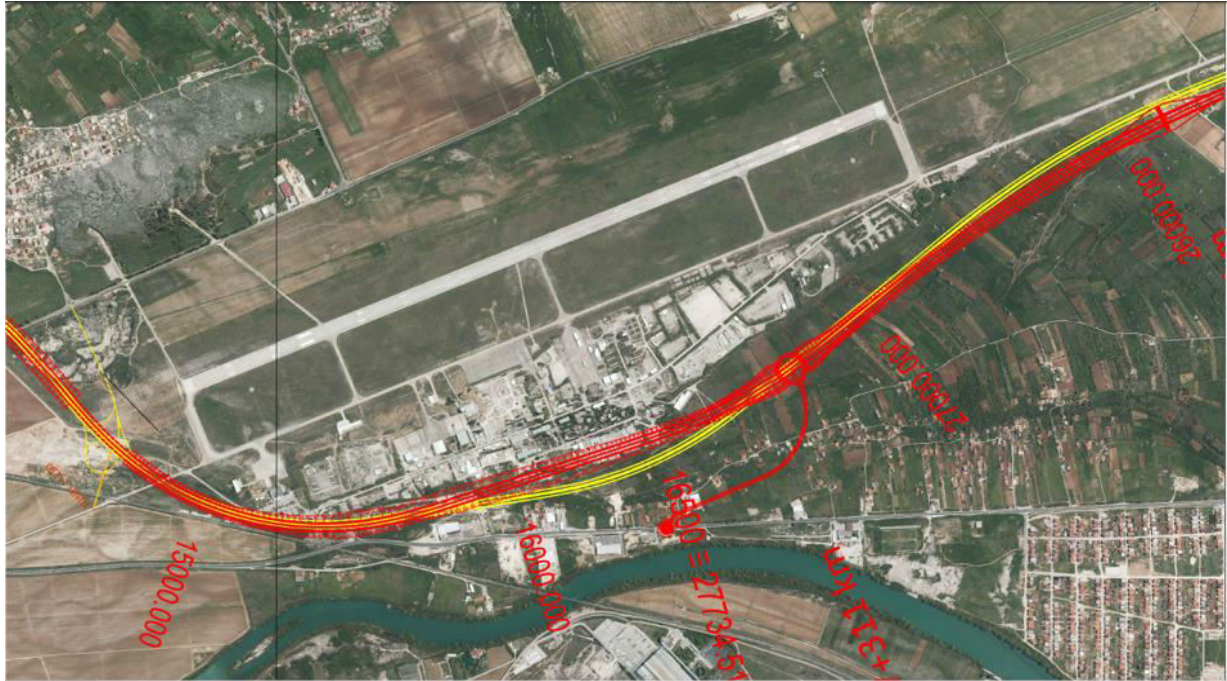
Figure 28: Initial alignment of the part of the section near the Mostar Airport passing over the hangars (2016)
