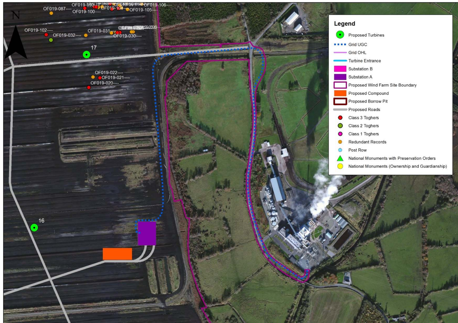
Figure 12-11 A: Archaeological constraints in north-east corner of site in relation to Substation Option A and associated grid underground cable route
