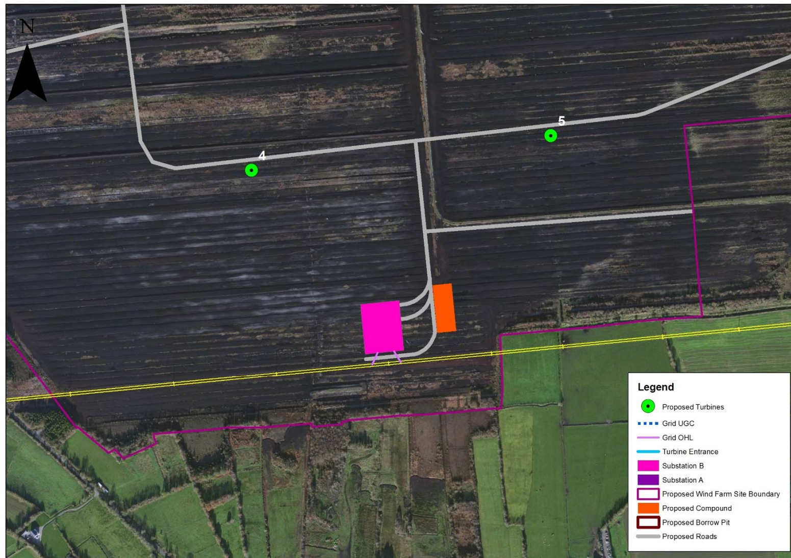
Figure 12- 11 B: Southern substation Option B and associated OHL connecting to existing electricity line
