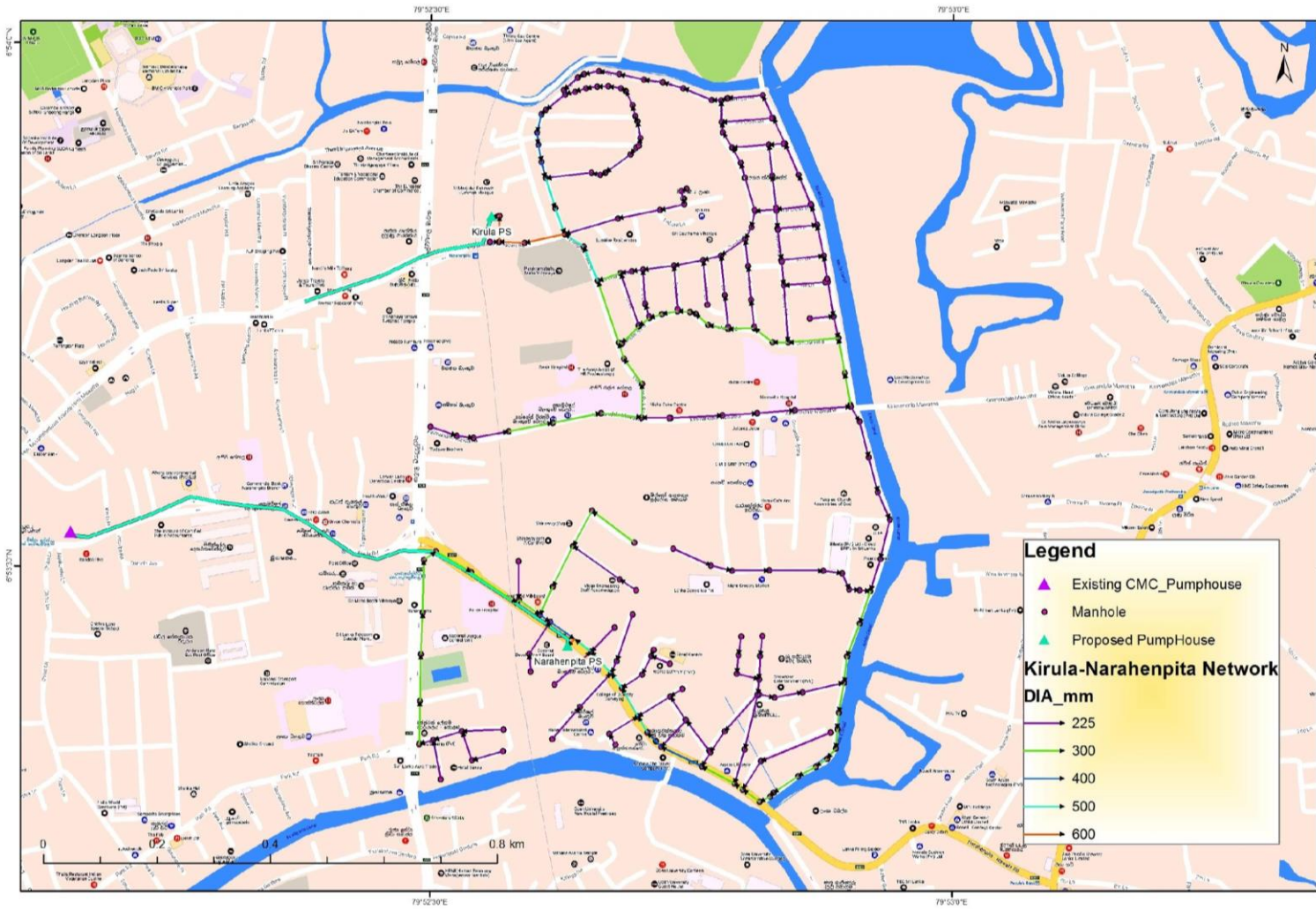
Figure 3.10 – Sewer network (variation of pipe diameter)
