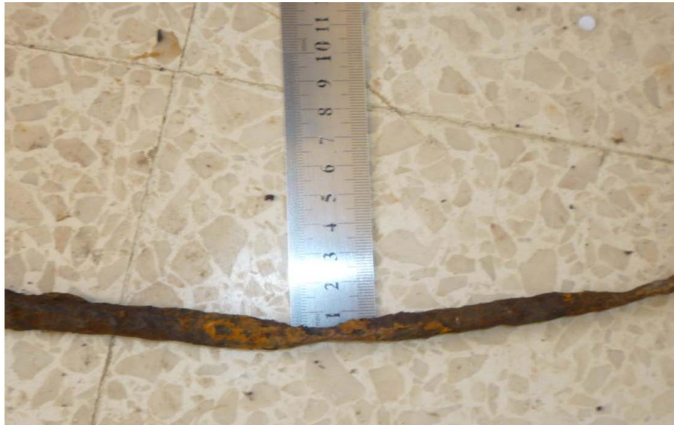
Plate 40: Loss of section in reinforcing steel
