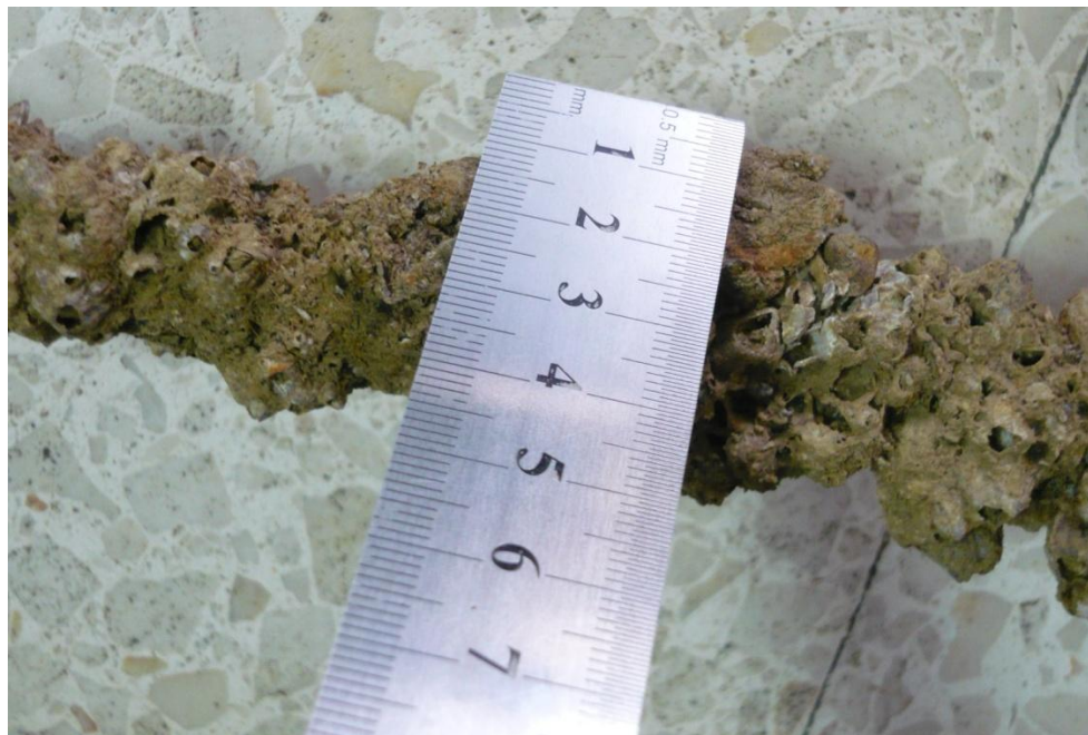
Plate 41: Incrustation on reinforcing steel
