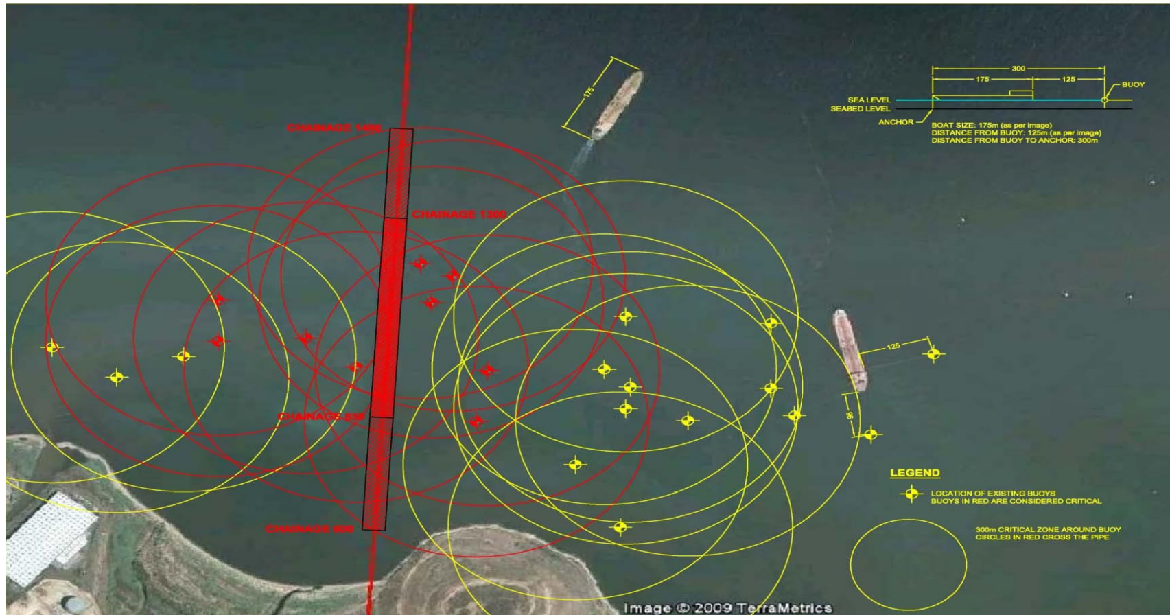
Plate 6: Critical buoys affecting the pipes
