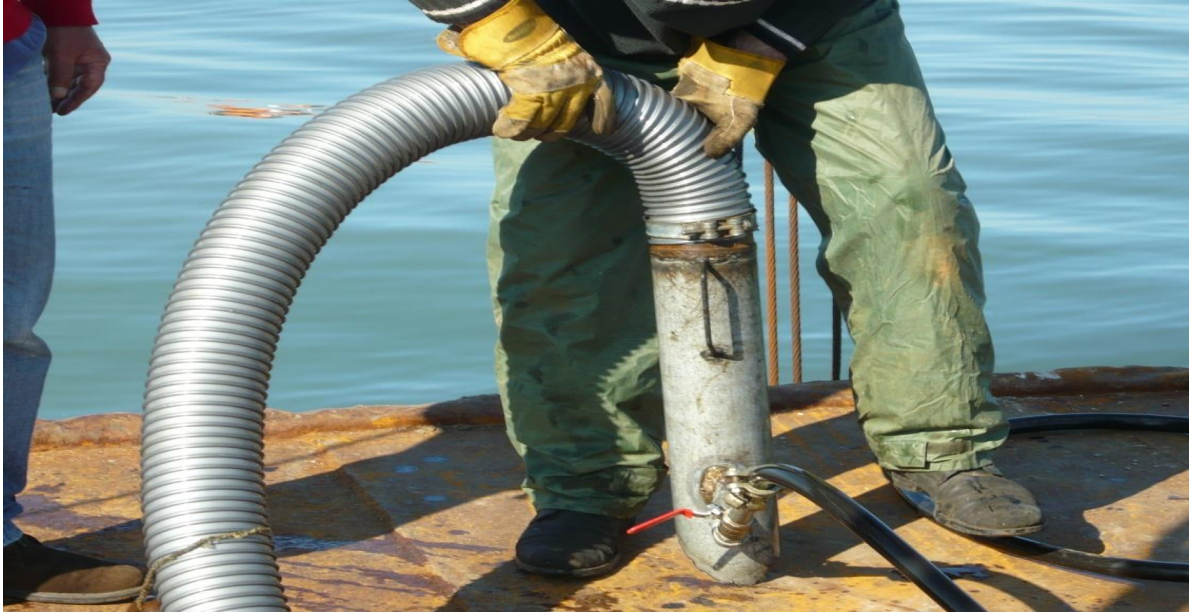
Plate 19: Air lifting nozzle
