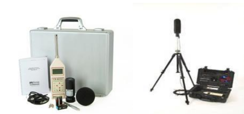
Figure 5-7 Sound Level Meter and Outdoor Measurement Kit Used in Noise Monitoring
