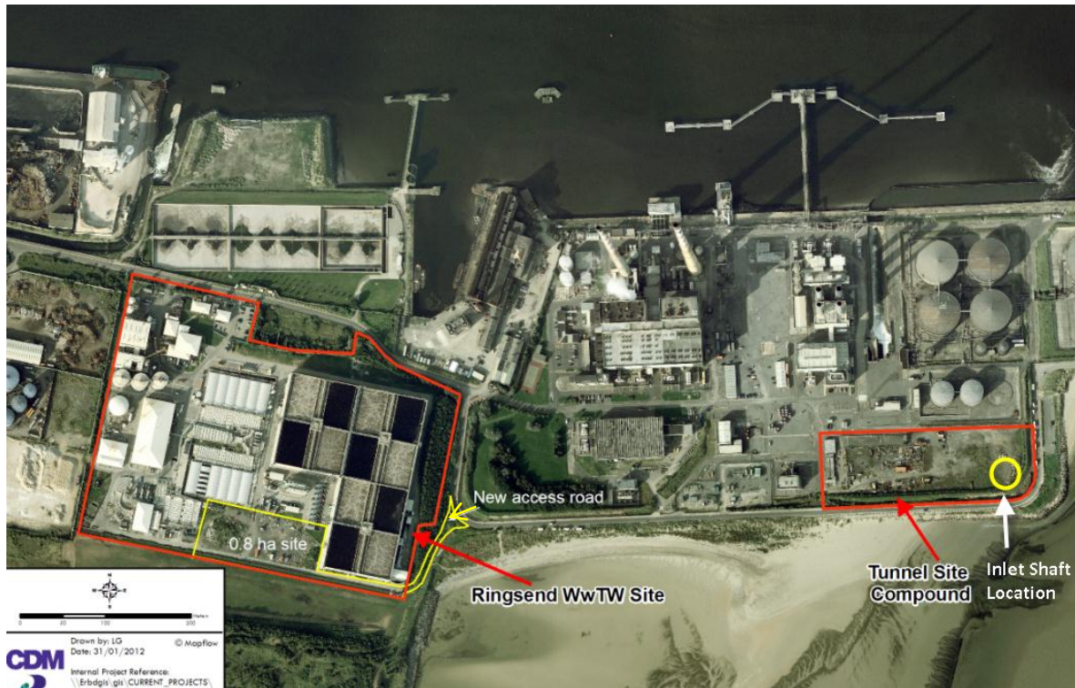
Figure 3 Ringsend WwTW and Tunnel Compound Site Locations (red) and open 0.8 ha space for construction (yellow rectangle)
