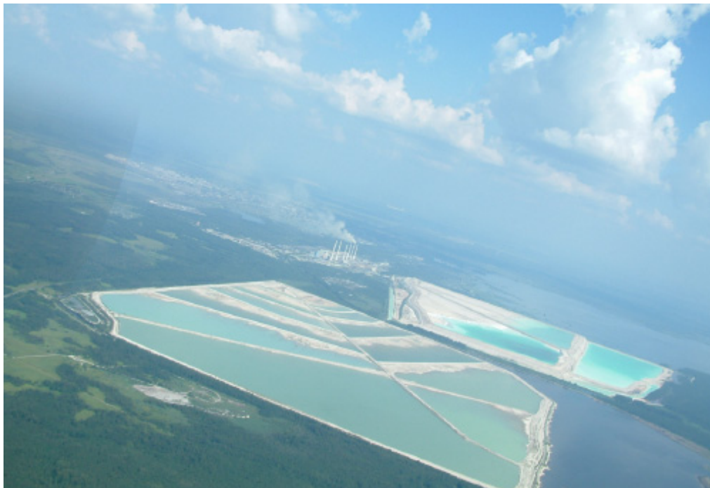
The ash field no 2 (in the front in approx. 2003). During planning and SEA process in 2006-2007 the closing process was active. Closing of ash field consists landscaping of territory, neutralisation of alkaline water etc to transform object harmlessly to environment.
