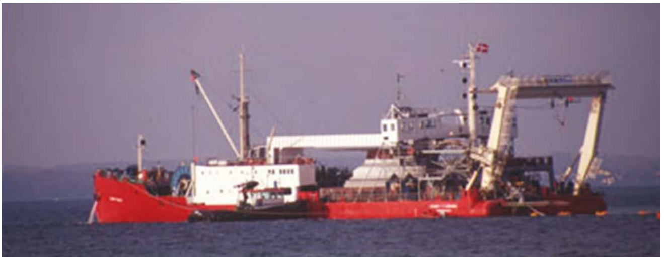
Figure 5: Typical Cable Lay Vessel (Source: Middelgrunden OWF)
