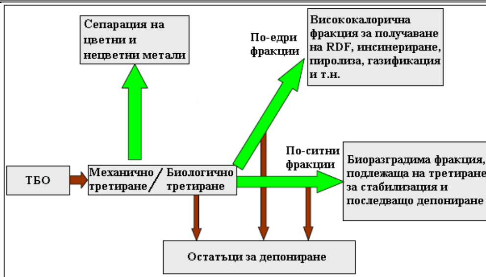
Fig. 2.2.2 Diagram of the incoming and outgoing streams in mechanical and biological treatment (the brown arrows show the path of residual materials and the green ones, the path of treated outgoing streams).
