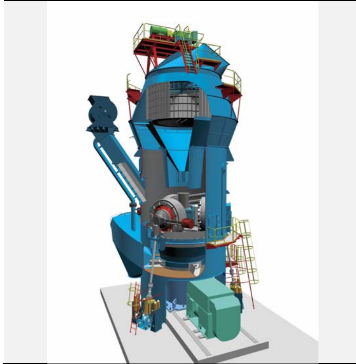
Figure 2-5 ATOX Vertical Roller Mill
