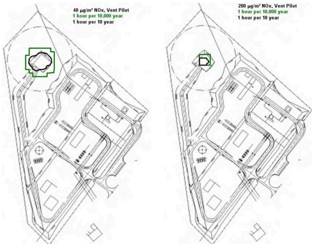
Figure 7-10 Left: Dispersion of NO x , 40 µg/m 3 , pilot burner, alternative vent system. Right: Dispersion of NO x , 200 µg/m 3 , pilot burner, alternative vent system.
